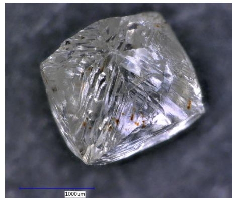
https://naturalsciencesresearch.wordpress.com/ "NCSM 5997. This octahedral diamond crystal looks like it has been faceted. These are all natural growth textures on the triangular crystal faces"
